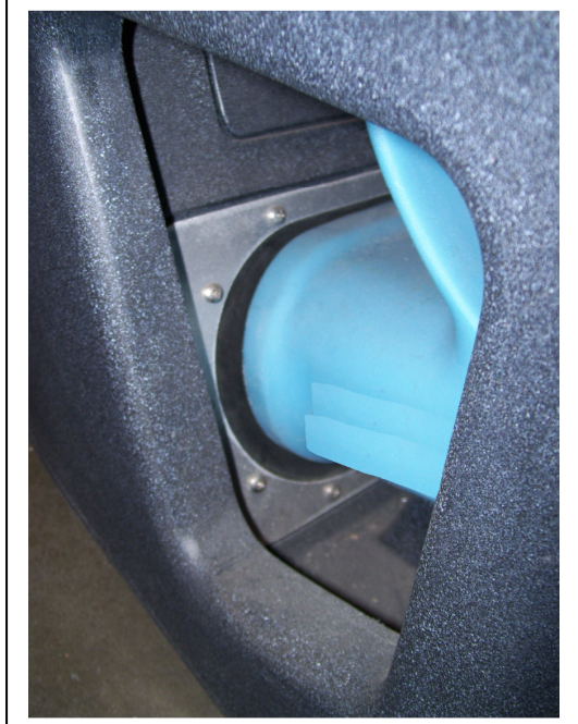
Short snout of air mover with large handle just barely sealed by E-TES SD gasket
