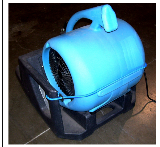
A bungee cord can be used to secure the air mover and maintain sufficient air flow
